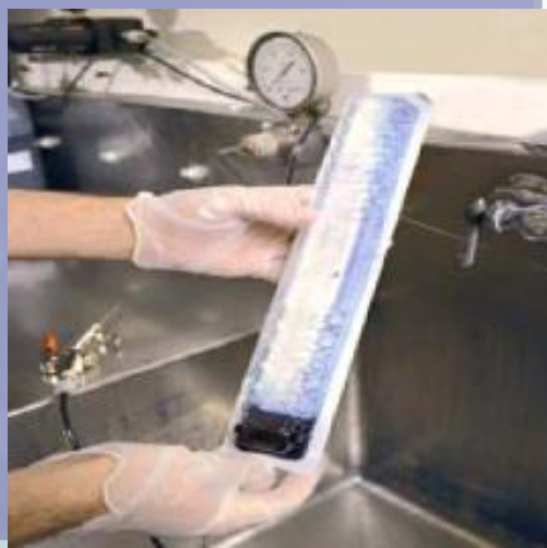
Dye Penetration Testing ASTM F 1929
